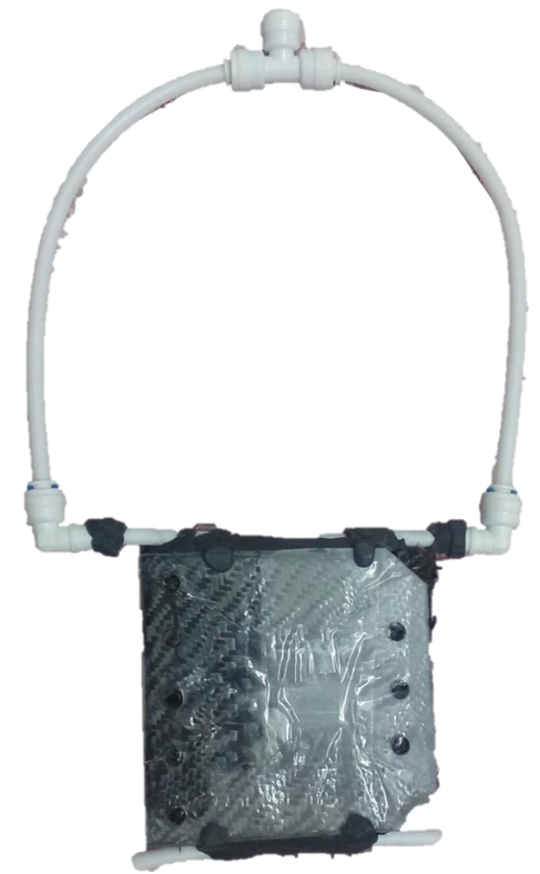
Working prototype of Capacitive De-Ionization unit
